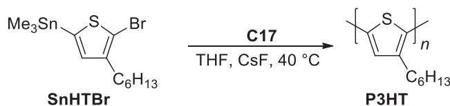
Scheme 7. Synthesis of poly(3-hexylthiophene) using a Pd–NHC catalyst.
