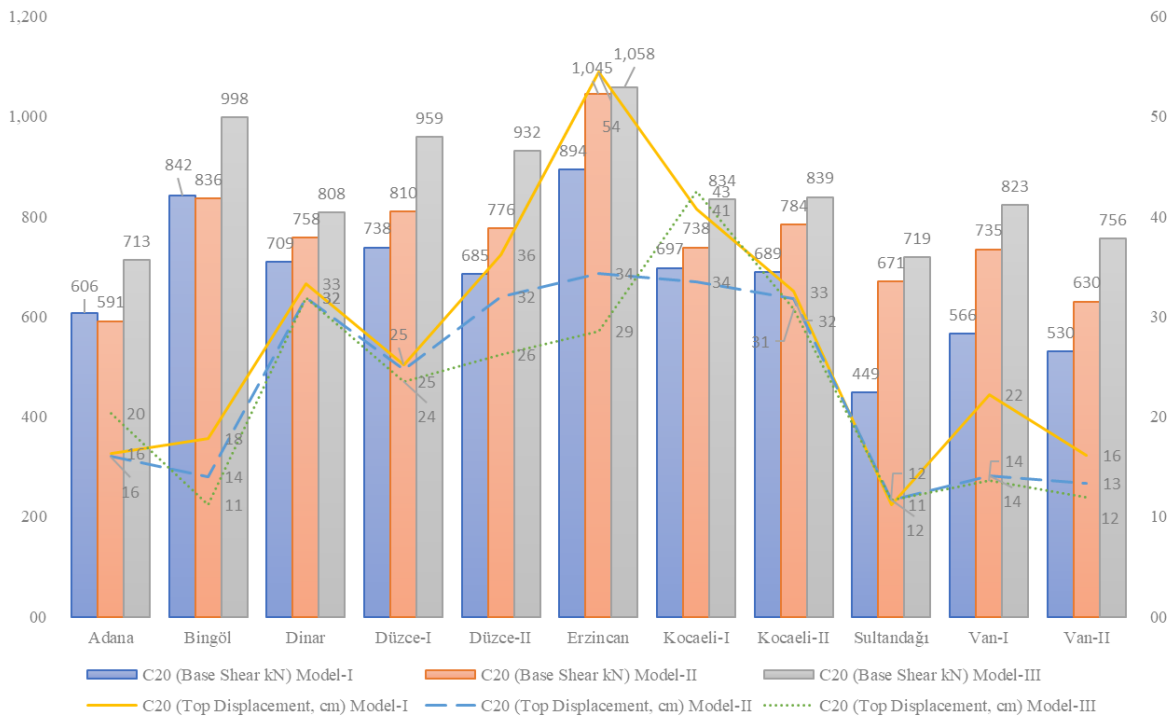
Figure 8: Seismic response of the seven-story generic numeric model with C20 concrete
