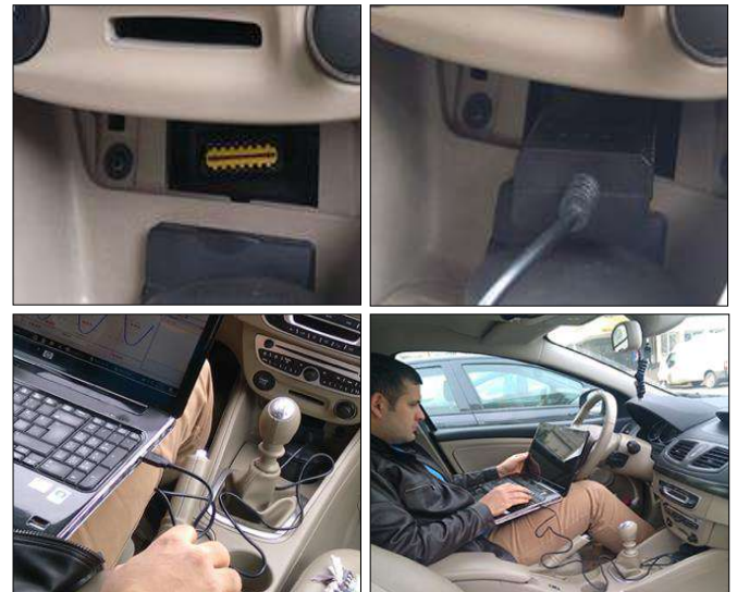
Figure 10. Data acquisition via OBDII
