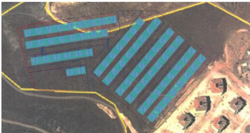
Figure 8. Excavation plan if the site is ripped
