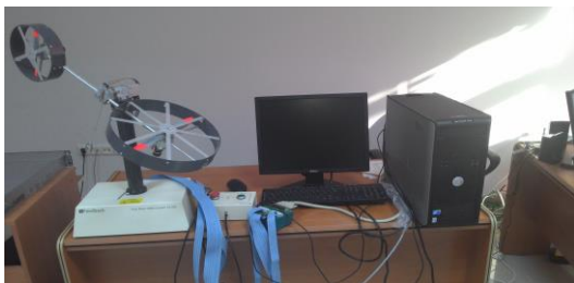
Fig. 8. TRMS Experimental Setup
